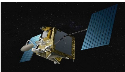
Each satellite is about a meter cubed and weighs less than 150kg
