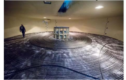
Picture 5: The Marea cable wound up inside the ship hold
